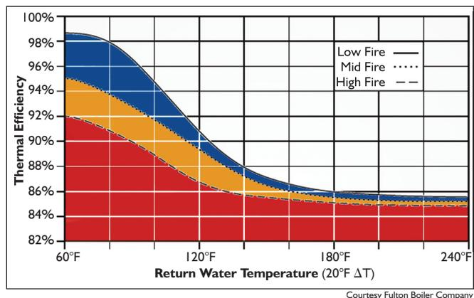
Figure 3: Thermal efficiency vs. return water temperature.
